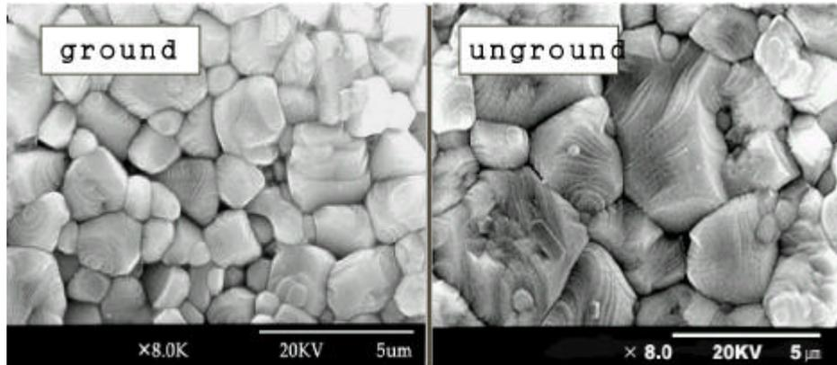
**Fig. 10.** SEM micrographs of  $\text{LaAlO}_3$  ceramics by unground and ground sintered at 1500 .
