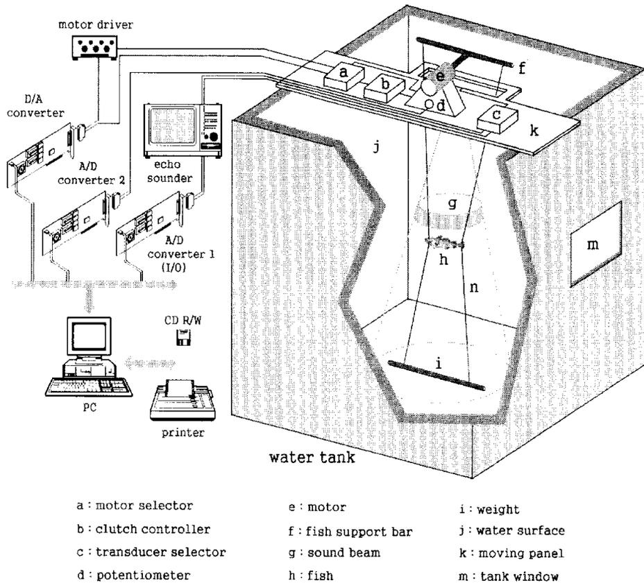
Fig. 1. Arrangement of experimental setup in water tank.
