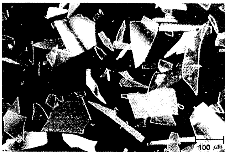
Photo. 15 Macro-graph of glass flake (thick : 3 \times 4 \mu\text{m} )
