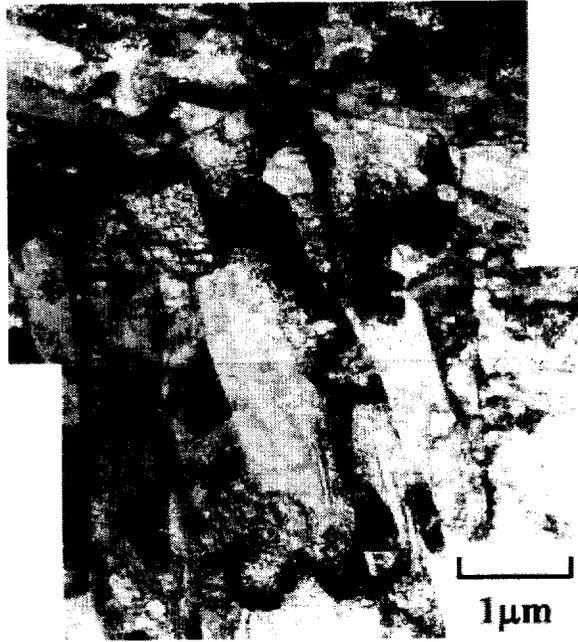
Fig 2.4.5 Transmission electron micrograph showing the lath martensite structure obtained from the specimen aged at 480°C for 1h
