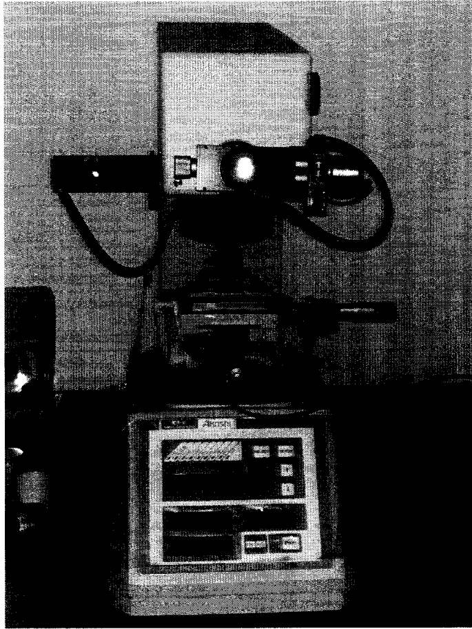
Fig. 11 Micro vickers hardness tester(MVK-H1)
