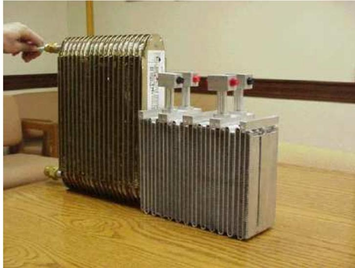
Photo. 1.1 Conventional (left) and prototype (right) CO<sub>2</sub> evaporator for mobile air-conditioner.
