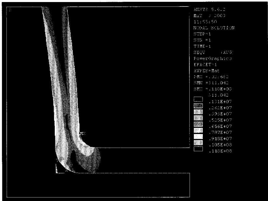
Fig. 9 Result of stress analysis at a stress concentration part of cross section
