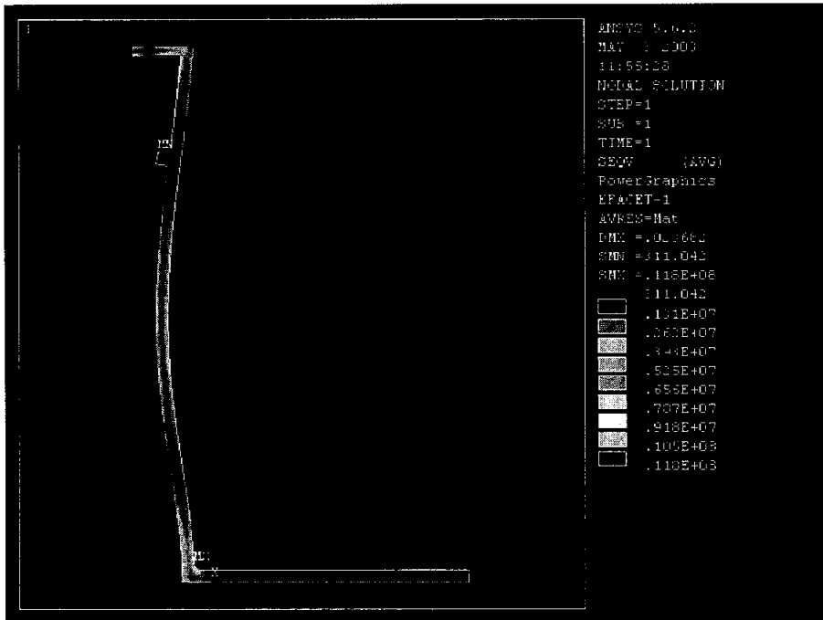
Fig. 8 Result of stress analysis at a cross section
