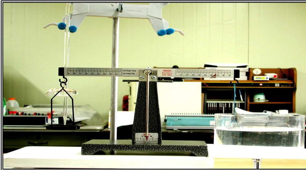
Photo 1 Surface tension measurement equipment
