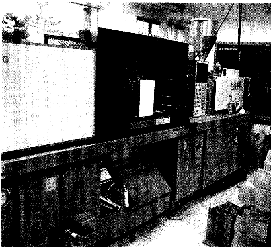
Photo 3 Injection Moulding Machine LG140N
