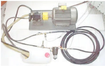
Fig. 3.3 Photo of test system for measuring steady state pressure loss in a spiral tube
