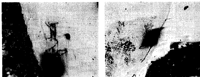
Fig. 3.13 The crack occurred from porosity and inclusion
