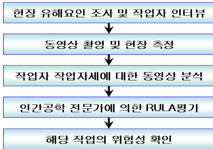
Fig. 11 Procedure of ergonomic analysis.
