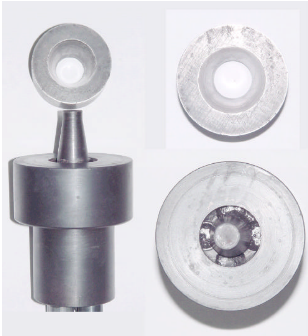
Fig. 11 The photograph of the conical dies and conical plug for the experiment
