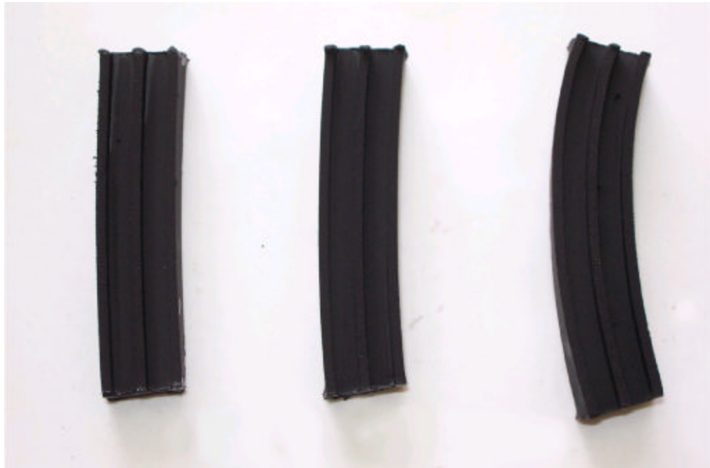
Fig. 8 The photograph of the curved square-tube with fin extruded by extru-bending process
