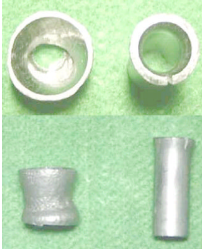
Fig. 22 The results of the expanding test by the compression in to the hole using conical punch
