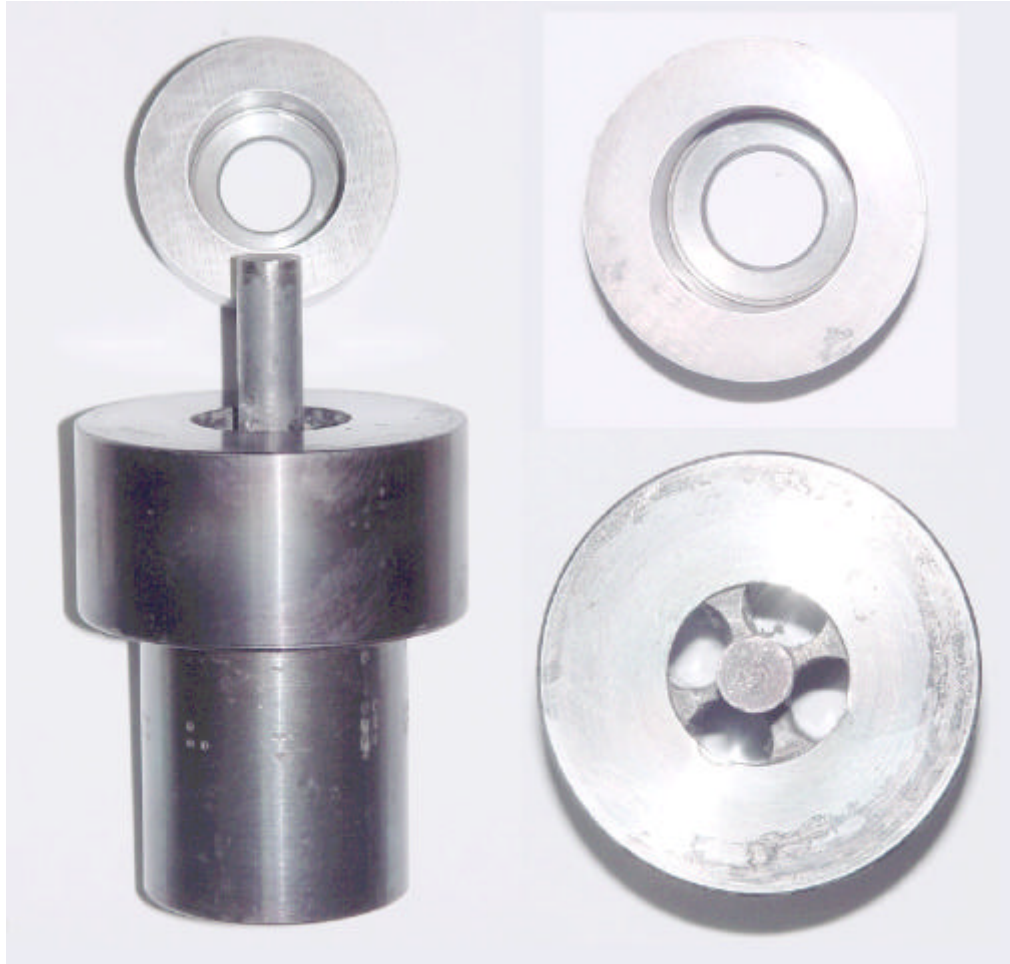
Fig. 14 The Photo of the flat dies and straight mandrel for the experiment
