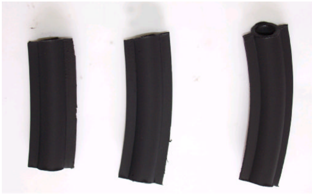
Fig. 7 The photograph of the curved circular-tube with fin extruded by extru-bending process
