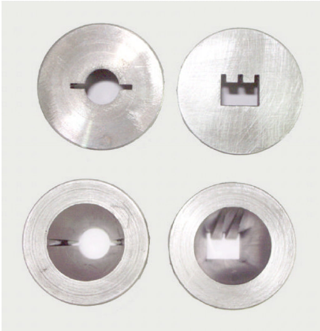
Fig. 3 The photograph of circular conical die with fin
