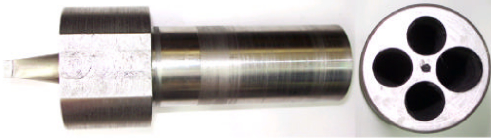
Fig. 5 The figure of circular conical plug with fin and multi-hole container with difference of hole diameters
