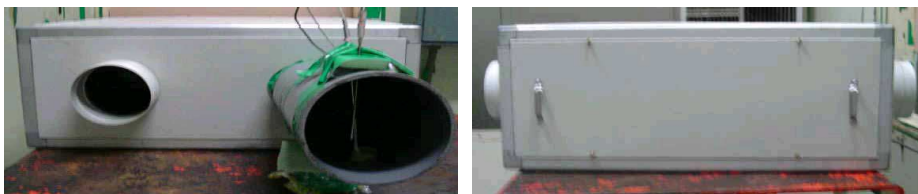
Fig. 30 C, Heat pipe type
