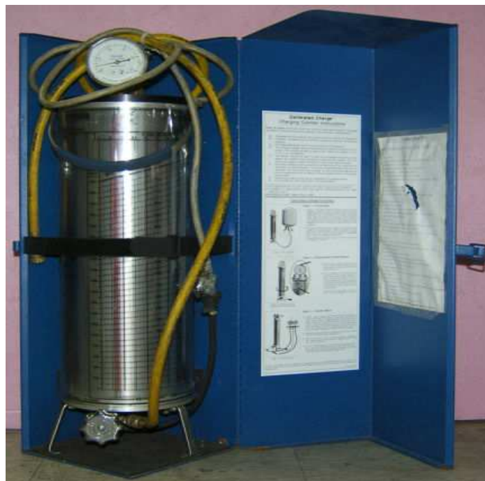
Fig. 16 Photograph of refrigerant charging cylinder
