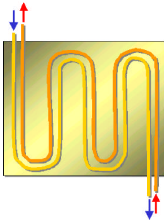
Figure 13. Design of Cu plate / Cu tube.
