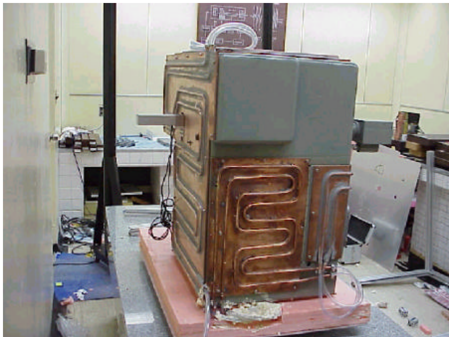
Figure 15 (a). Gauge block interferometer being modified.
