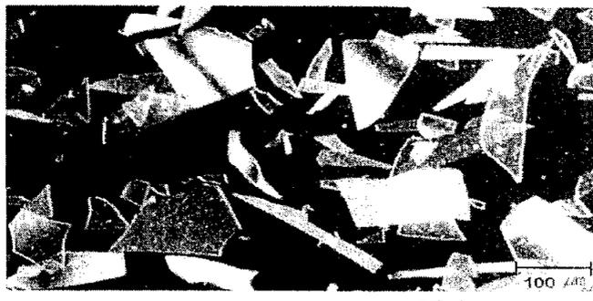
Photo. 2 Macro-graph of glass flake (thick :  $3 \times 4 \mu\text{m}$ )
