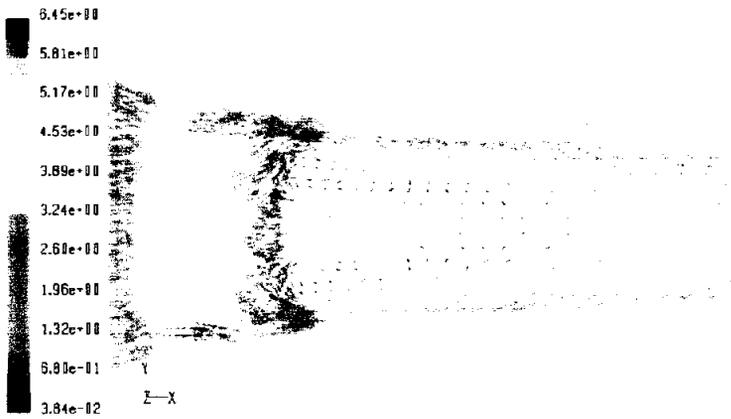
Fig. 4.29 Velocity vectors at T-junction
