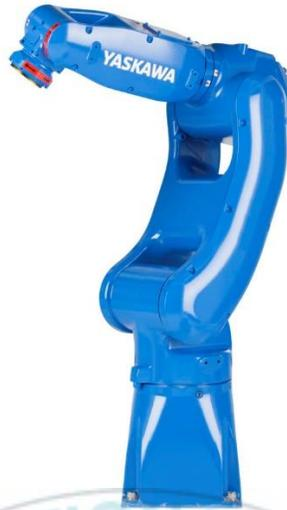
**Figure 3 Robot Motoman Yaskawa-GP8 <sup>1</sup>**
