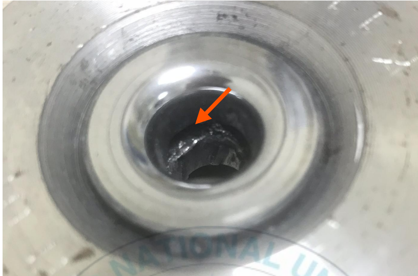
Fig. 4.1 Image of broken drawing die
