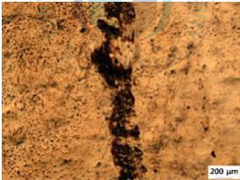
Fig. 3.6 Shapes of wear tests with VC layer
