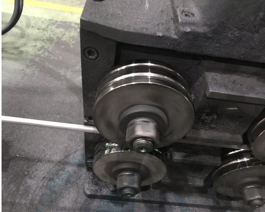
Fig. 3.12 VC coated pinch roller at High frequency induction heat treatment equipment
