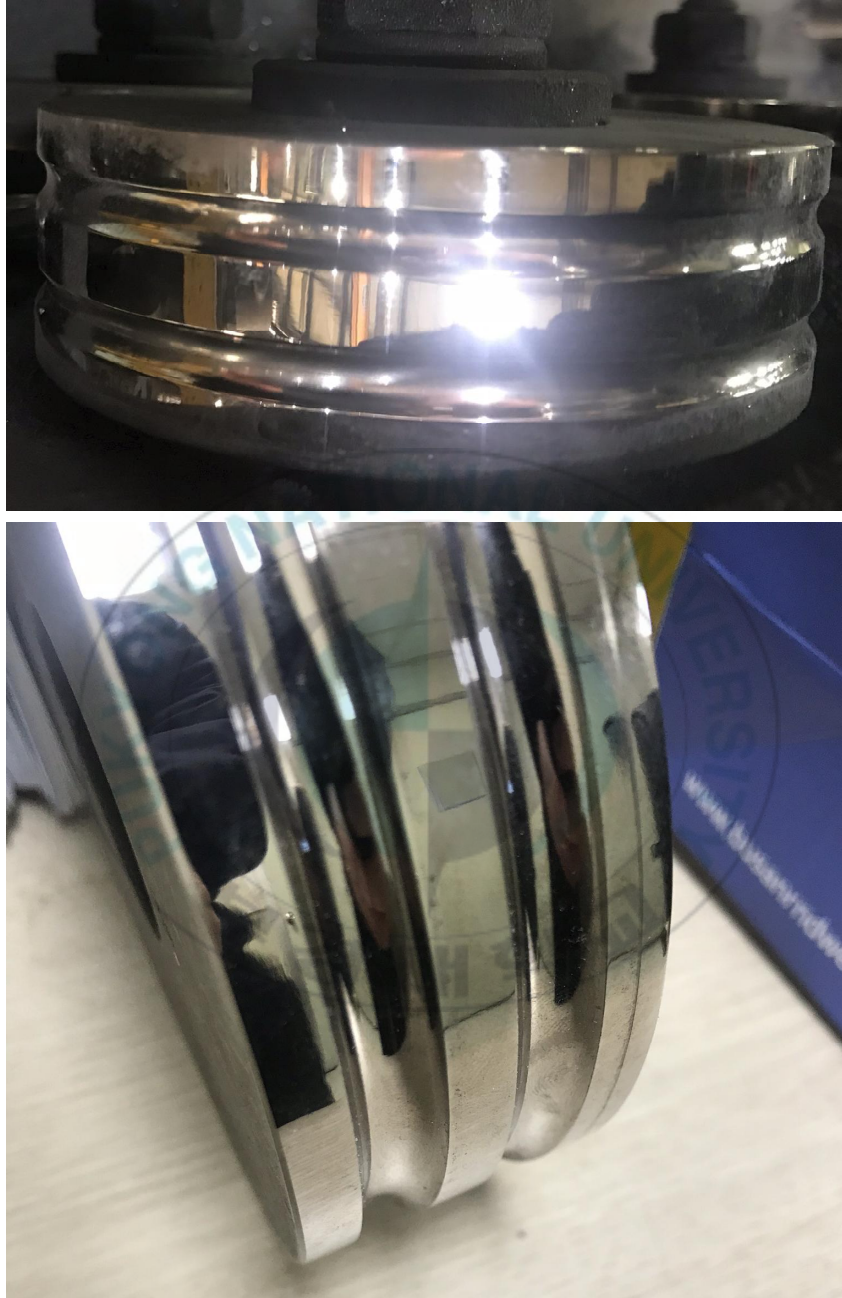
Fig. 3.3 VC coated pinch roller
