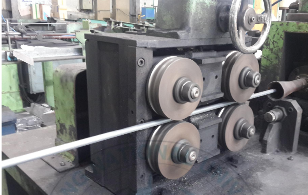
Fig. 3.2 Pinch roller at High frequency induction heat treatment equipment
