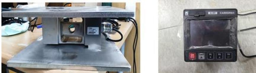
Fig. 7 Experiment tools : load cell and Indicator
