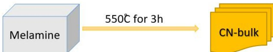
Figure 2.1 Scheme of synthesis CN-bulk
