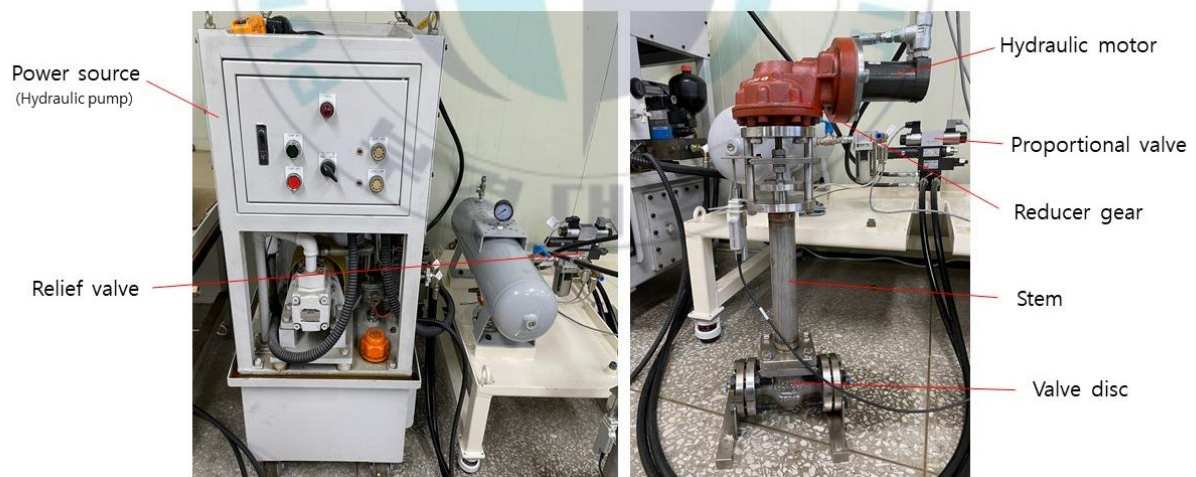
Fig. 4-1 ESD valve system experimental equipment
