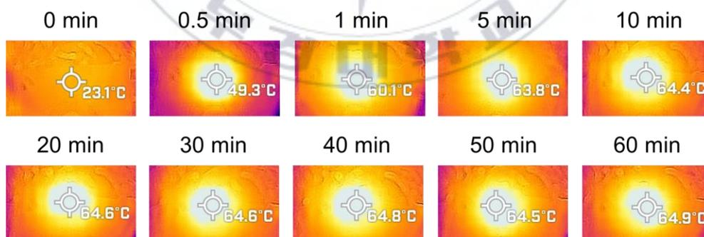
**Figure 10.** Infrared image of the paper-based device patterned with the carbon-black-PDMS. The sample loading disc located in the center of the paper-based device showed stable temperatures for 1 hour.
