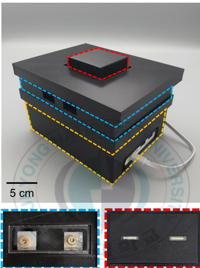
**Figure 15.** Photo of the laser-diode device. Laser-diode device consists of three floors. The first floor (yellow line) contains laser-diode circuit, Arduino UNO, and portable battery. The second floor (blue line) contains two laser diodes and two fans. Third floor (red line) contains the paper-based device with the anti-evaporation case.
