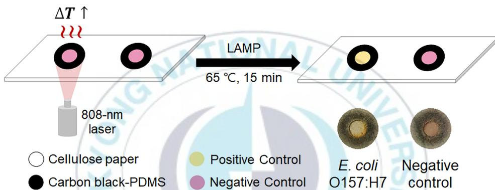
**Figure 5.** Overview of carbon-black-PDMS patterned paper-based device. Using the heat generated by a photothermal effect of carbon-black and 808-nm laser, LAMP was conducted to amplify *rfbE* gene of a foodborne pathogen *E. coli* O157:H7
