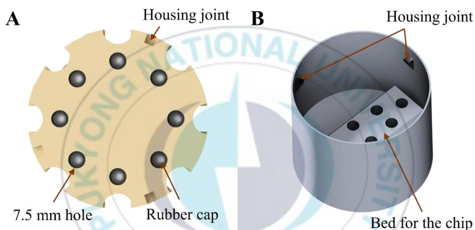
**Figure 12.** 3D illustration of the (A) bottom of the cartridge and (B) the cartridge without the tube holder and chip. The tube array consists of eight 7.5 mm holes at eight tubes' positions. When the chip's needles stab the vacutainer stoppers, reagents inside one tube will be steered toward another through the silica matrix inside the chip. The tube array has three housing joints which help the tube array fix to the cartridge.
