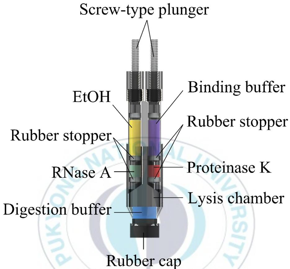
**Figure 9.** CAD design showing sectional view of the compartmentalized tube consisting of lysis reagents including digestion buffer, proteinase K, Rnase A, EtOH and binding buffer. These buffers are pre-loaded in compartmentalized chambers and can be released by rotating the screw-type plungers.
