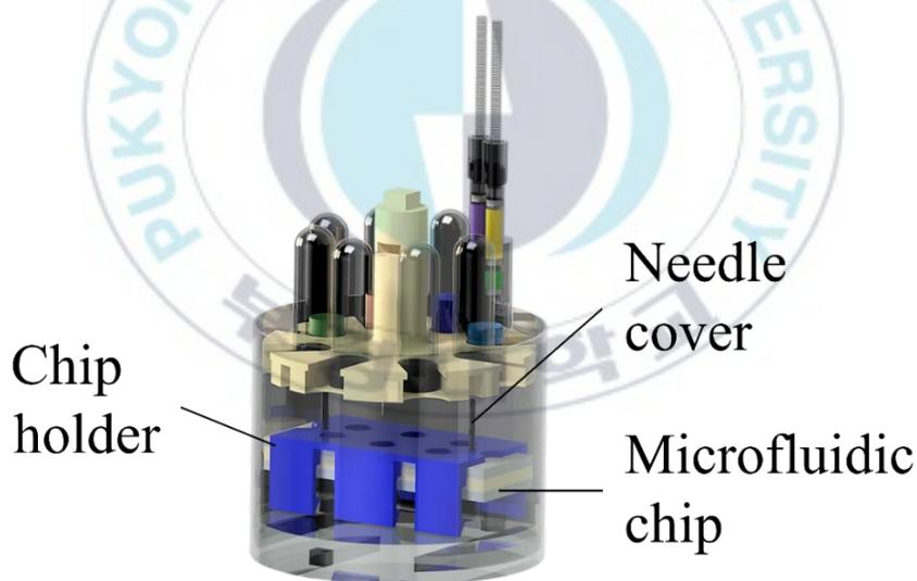
**Figure 11.** CAD design of the cartridge comprising the chip and the tube holder.
