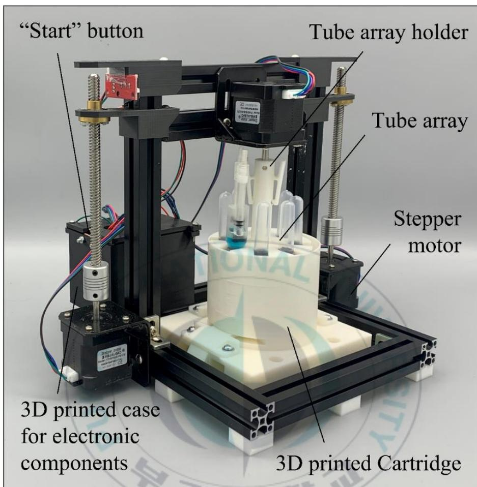
**Figure 14.** An automated silica-based DNA purification machine utilizing a closed-system pressurized cartridge for bacteria extraction.
