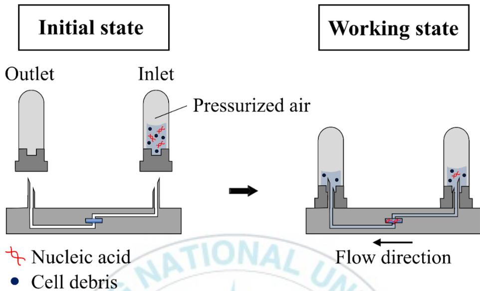
**Figure 1.** Schematic illustration of the working concept of the chip. At the initial state, the reagent is pre-loaded. At the working state, the tubes' septum are stabbed by the needles of the microfluidic chip which will allow pressurized air to transfer the reagent from the inlet to the outlet without using any external hardware to manipulate the fluid flow.
