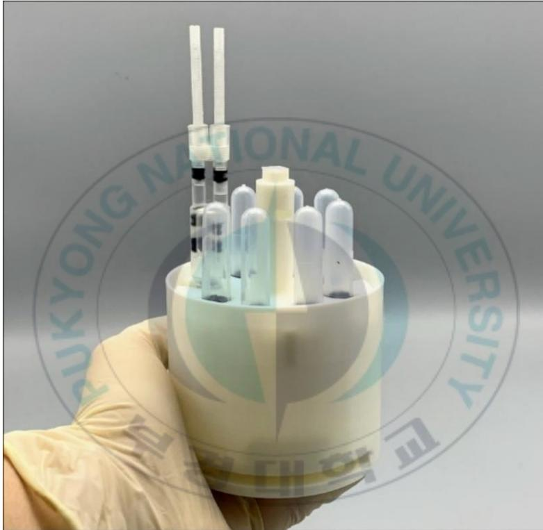
**Figure 13.** Digital image of the 3D printed cartridge.
