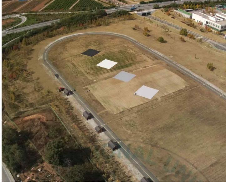
Figure 2 The site of fieldwork and the tarps installed on the site
