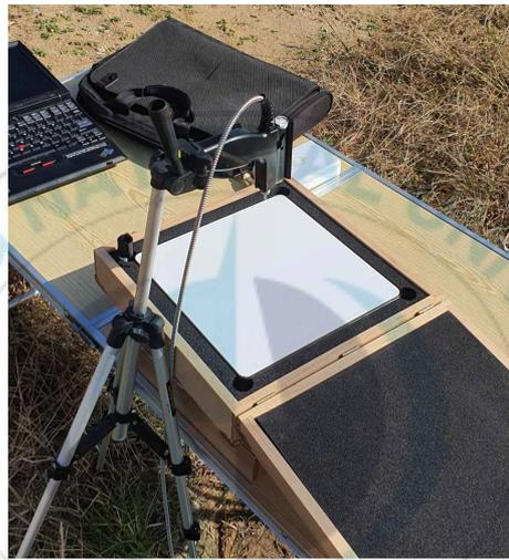
Figure 8 The spectral white reference(WR) and spectroradiometer
