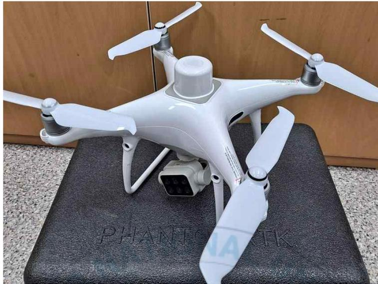
Figure 3 P4 Multispectral
