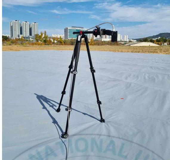
Figure 9 The spectroradiometer measuring radiance of tarps
