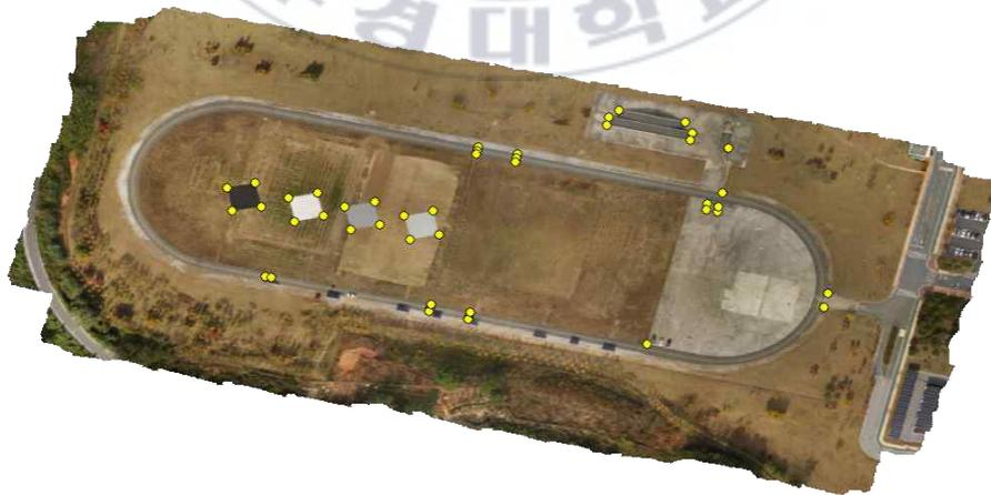
Figure 6 Location of ground control points(GCPs)
