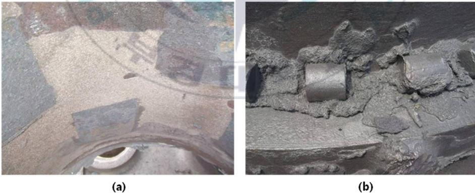
Fig. 4. Example of sand burn-on and sand burn-in of foundry sand
