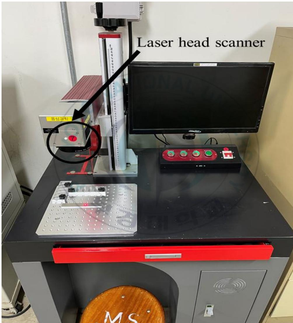
**Fig. 8** Photo of the laser-engraving machine.
