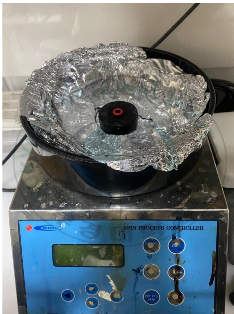
Figure 7. Spin coater in our LAB
