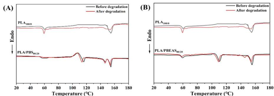
**Figure 21.** DSC curves of the (A) PLA and PLA/PBS (80/20) blends and (B) PLA and PLA/PBEAS (80/20) blends before and after degradation in the presence of an alkaline medium.
