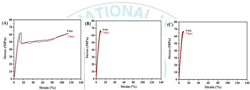
**Figure 15.** Stress-strain curves of (A) LOTTE-PC, (B) D-PC, and (C) SY-PC after Proteinase K enzymatic exposure for 7 days.
