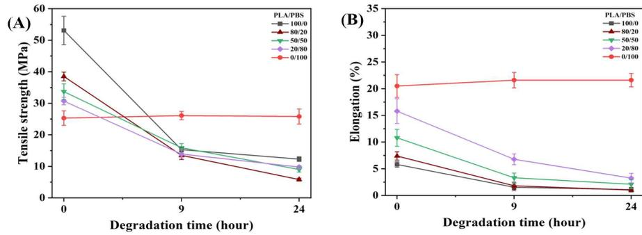
Figure 24. (A) Tensile strength and (B) elongation of PLA/PBS blends with various degradation times in the Tris-buffer solution containing 1 mg of Proteinase K.
