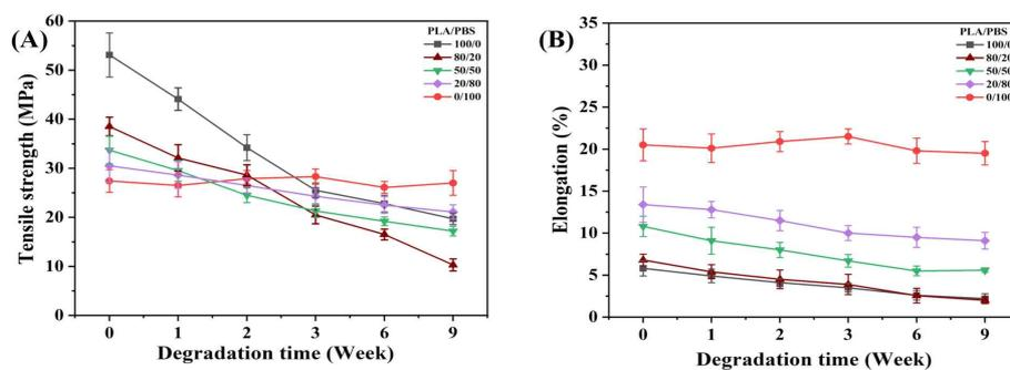
Figure 19. (A) Tensile strength and (B) elongation of PLA/PBS blends with various degradation times in the presence of an alkaline medium at pH 11.
