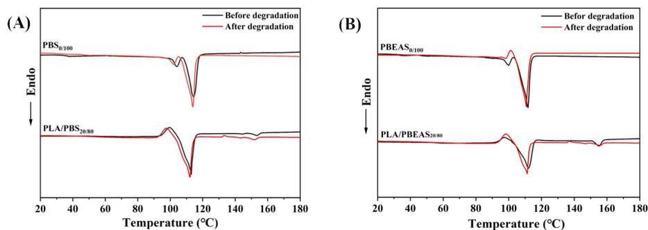
**Figure 29.** DSC curves of the (A) PBS and PLA/PBS (20/80) blends and (B) PBEAS and PLA/PBEAS (20/80) blends before and after degradation in the presence of Lipase.
