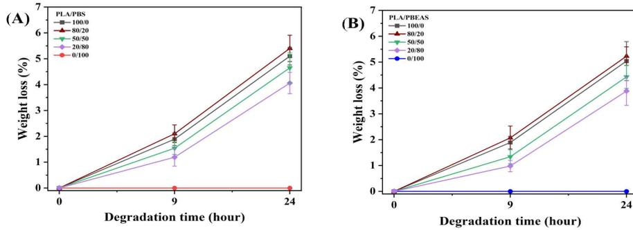
Figure 22. Changes in weight loss of (A) PLA/PBS and (B) PLA/PBEAS blends as a function of degradation times in the Tris-buffer solution containing 1 mg of Proteinase K.
