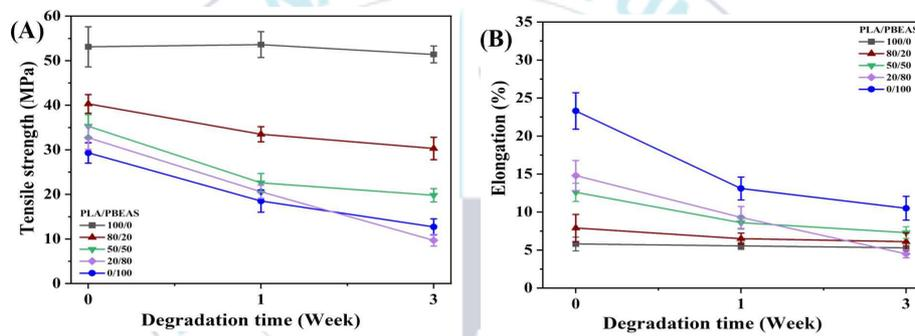
Figure 27. (A) Tensile strength and (B) elongation of PLA/PBEAS blends with various degradation times in the Phosphate buffer solution containing 3 mg of Lipase.
