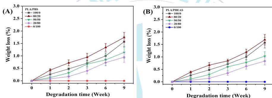
**Figure 18.** Changes in weight loss of (A) PLA/PBS and (B) PLA/PBEAS blends as a function of degradation times in the presence of an alkaline medium at pH 11.
