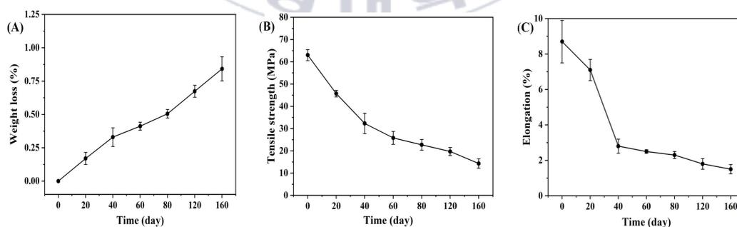
**Figure 16.** (A) % weight loss, (B) tensile strength, and (C) elongation of SY-PC as a function of degradation time in soil burial test.
