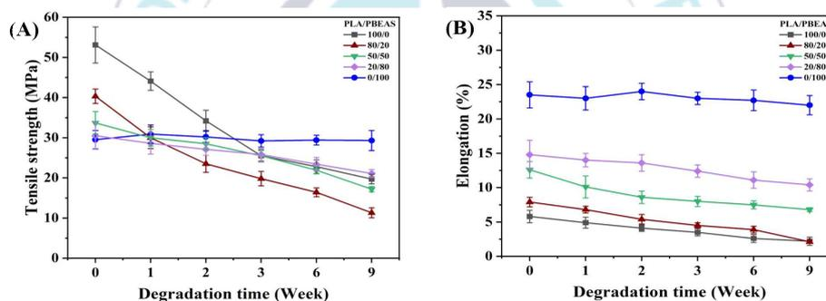
Figure 20. (A) Tensile strength and (B) elongation of PLA/PBEAS blends with various degradation times in the presence of an alkaline medium at pH 11.
