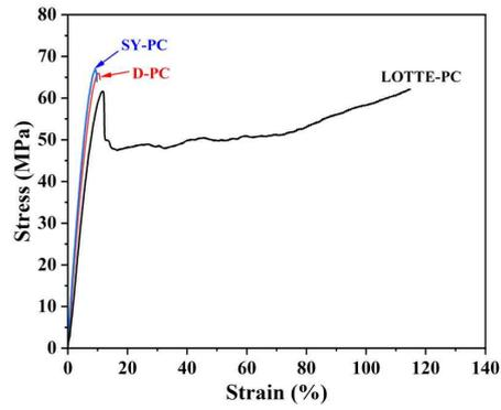
Figure 13. Example of stress-strain curves of PCs.
