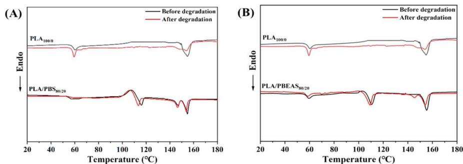
**Figure 28.** DSC curves of the (A) PLA and PLA/PBS (80/20) blends and (B) PLA and PLA/PBEAS (80/20) blends before and after degradation in the presence of Proteinase K.
