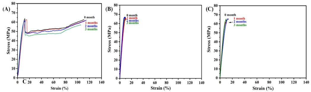
**Figure 14.** Stress-strain curves of (A) LOTTE-PC, (B) D-PC, and (C) SY-PC after alkaline exposure for 3 months.
