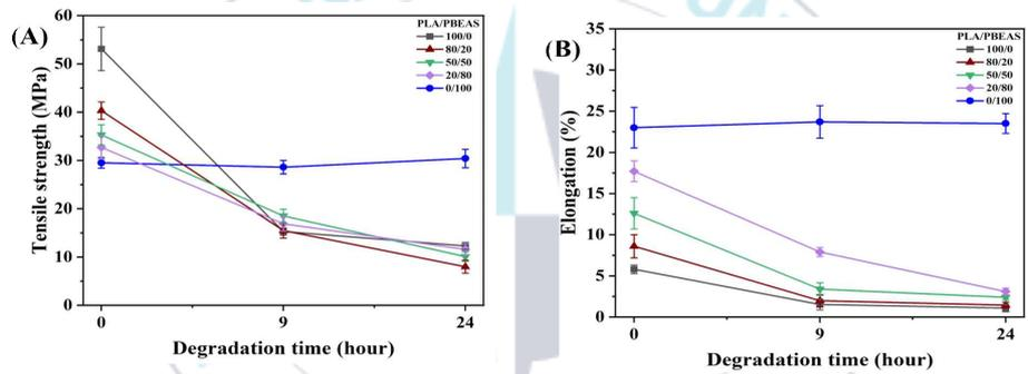
Figure 25. (A) Tensile strength and (B) elongation of PLA/PBEAS blends with various degradation times in the Tris-buffer solution containing 1 mg of Proteinase K.
