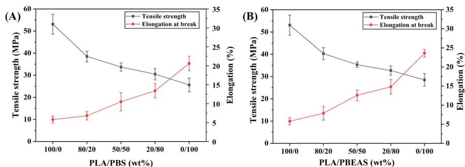
Figure 17. Tensile strength and elongation of the (A) PLA/PBS and (B) PLA/PBEAS blends before degradation.
