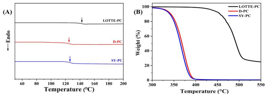
Figure 12. (A) DSC and (B) TGA curves of PCs. (The arrows indicate Tg)
