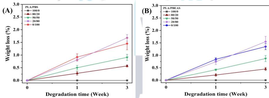
Figure 23. Changes in weight loss of (A) PLA/PBS and (B) PLA/PBEAS blends as a function of degradation times in the Phosphate buffer solution containing 3 mg of Lipase.
