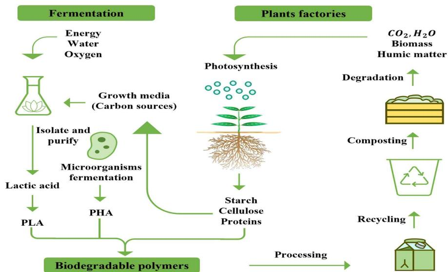
Figure 2. Cyclic biological process of biodegradable polymers [5].
