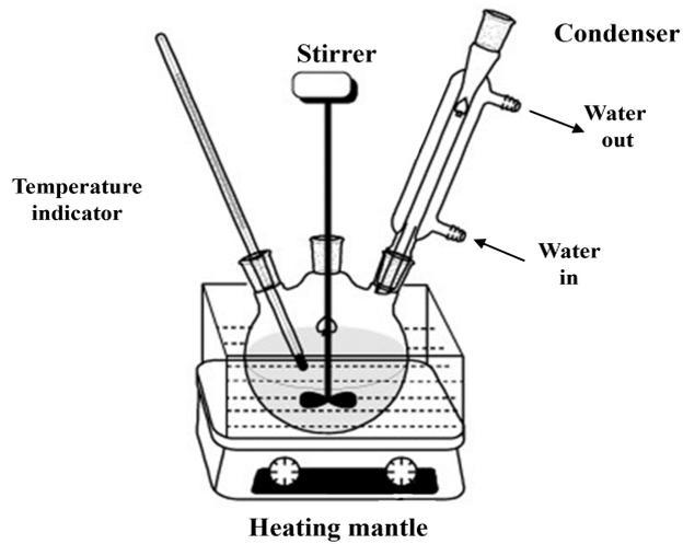
Figure 7. Synthetic tools for PLA polymerization.
