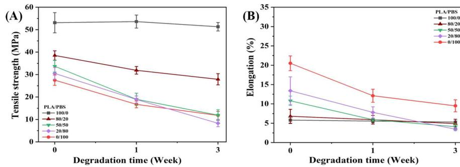
Figure 26. (A) Tensile strength and (B) elongation of PLA/PBS blends with various degradation times in the Phosphate buffer solution containing 3 mg of Lipase.
