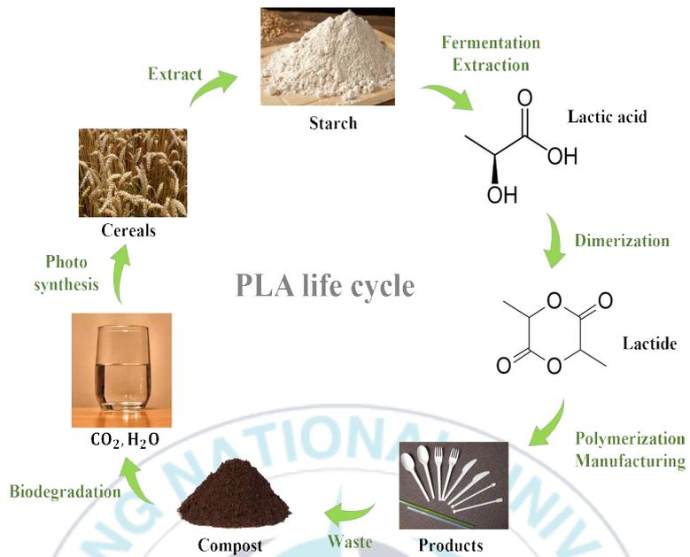
Figure 5. Schematic representation of PLA production [27].
