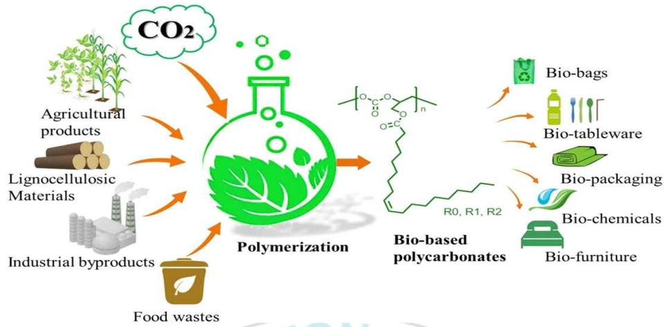
Figure 4. Bio-based polycarbonate is manufactured from a wide range of bio-based raw materials and CO<sub>2</sub> [25].
