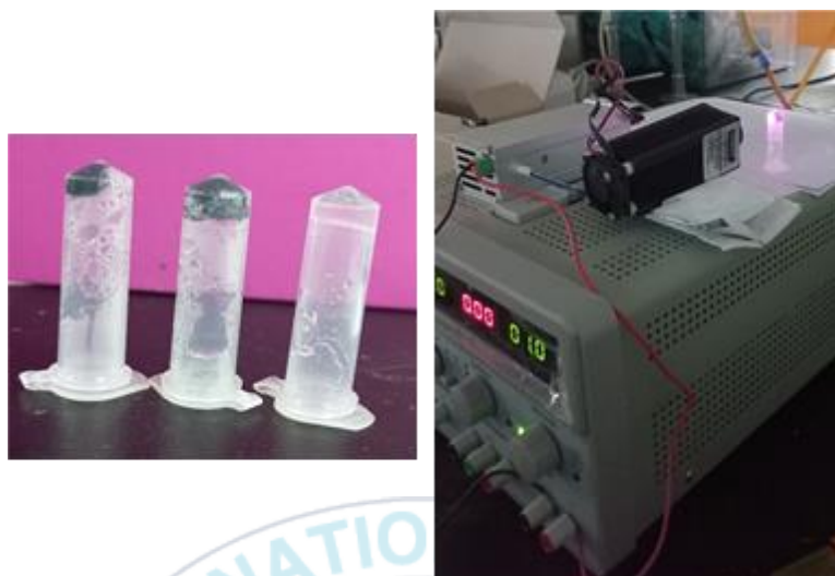
Fig. 31 Photothermal effect of NIR irradiation on hydrogels
