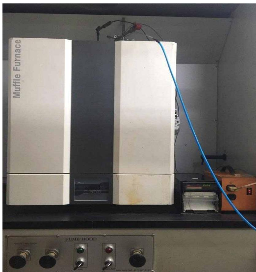
Photo 2. Experimental apparatus for spontaneous ignition temperature measurement.
