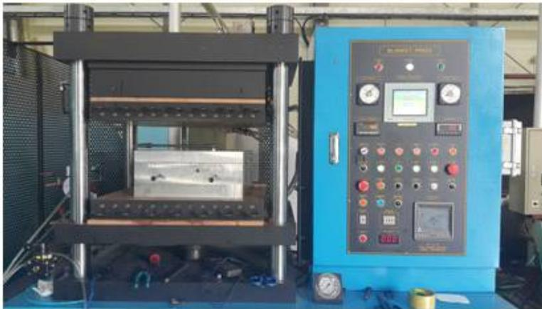
Figure 38 Press for RTM process.
