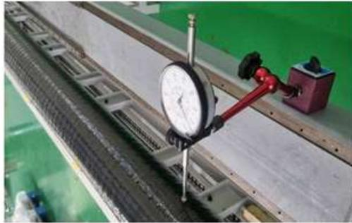
Figure 34 Deflection measurement of a composite tube.
