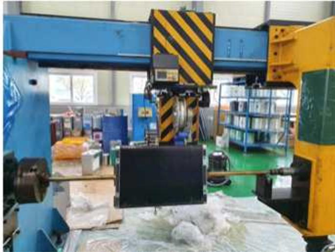
Figure 11 Winding of a UD composite plate.
