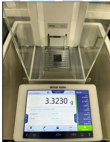
Figure 13 Measurement of composite sample weight using a precision balance.
