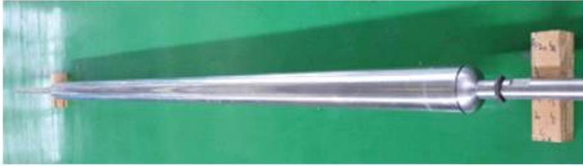
Figure 8 Mandrel for filament winding.
