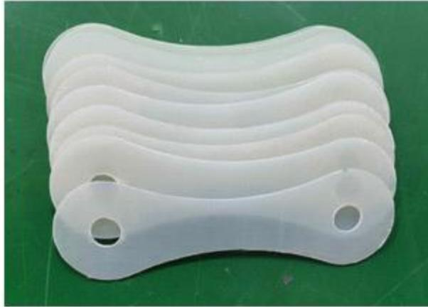
Figure 37 Sheets of laminated prepreg for disc pack manufacturing.
