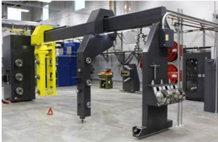
Figure 7 Typical filament winding machine.
