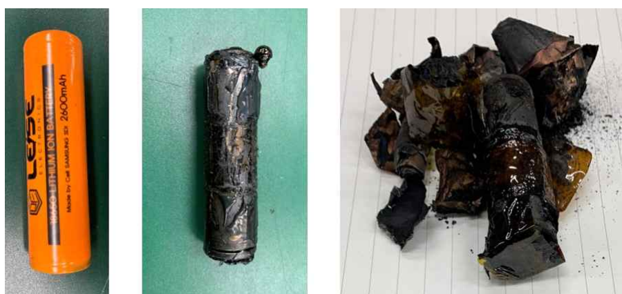
Figure 18 Picture of Samples (a) samples of before the experimental, (b) no-explosion case in the experimental results (c) explosion case in the experimental results.
