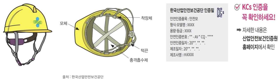
출처 : 한국산업안전보건공단 Fig. 1 Safety helmet shape and indication of safety certification
