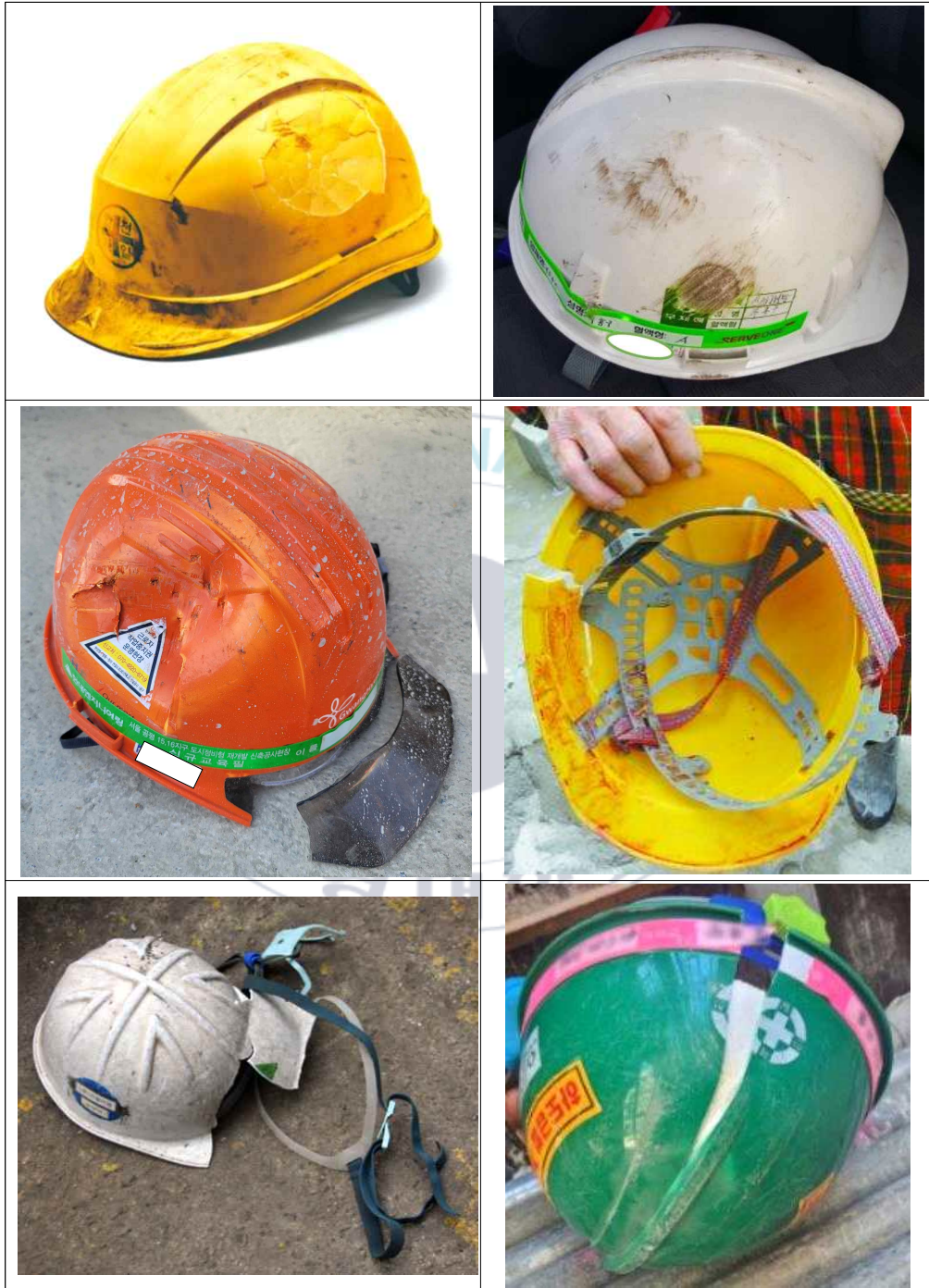
Fig. 9 The impact area on the safety helmet from the accident
