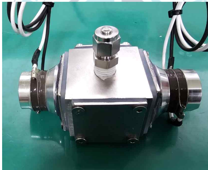
Fig. 3.5. Plenum chamber assembly.
