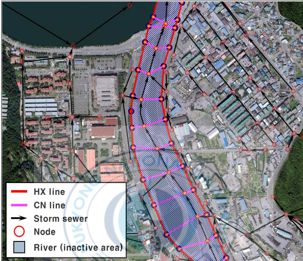
Fig. 5.2. The XP-SWMM models for Hx line and CN line.
