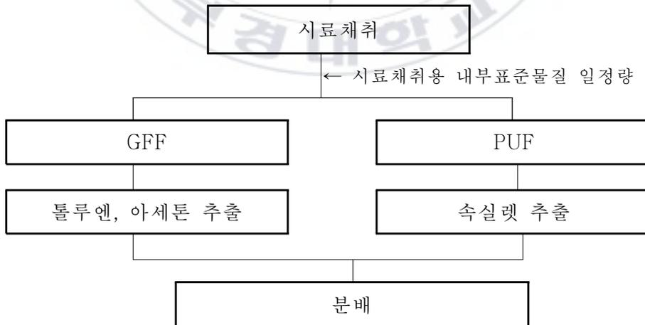
Fig.3-3. Diagram for extraction of samples.
