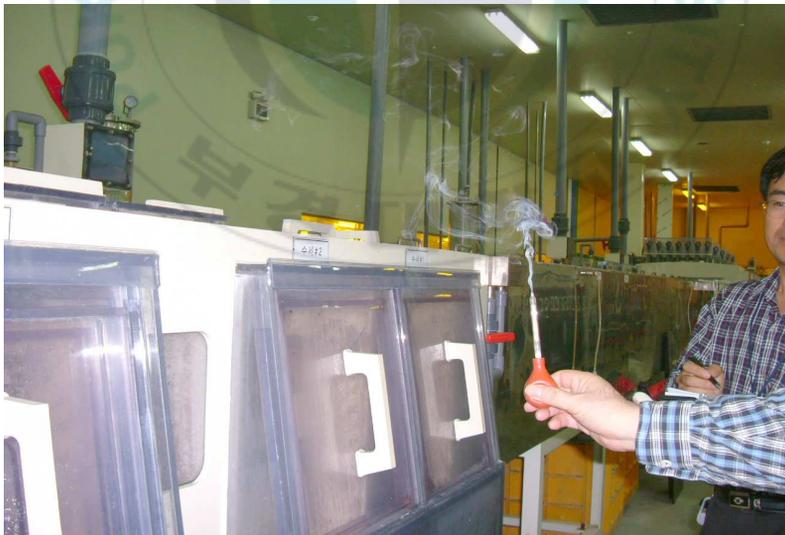
Fig. 4.12 Snapshot of Measurement (Air flow)
