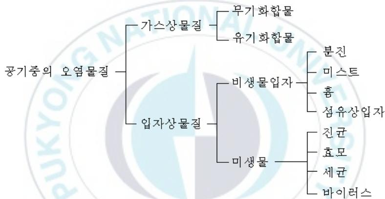
Fig. 2.2 Contaminant classification in air (加筆)
