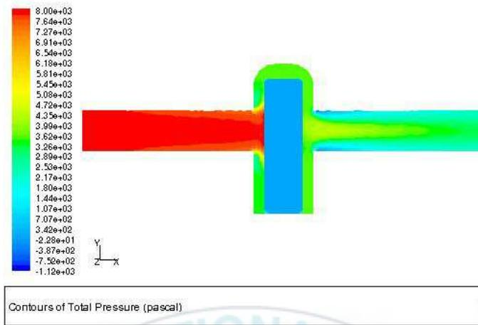
Fig. 2.20 Total pressure distribution at the central vertical section ( $z = 0$ )
