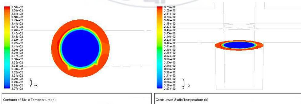
Fig. 2.15 Temperature distribution at section  $y = -10\text{mm}$
