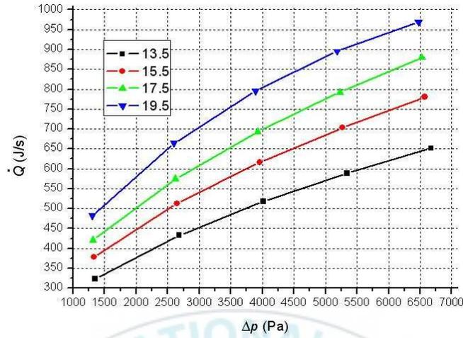
Fig. 3.11 Pressure difference  $\Delta p$  (Pa) vs. heat transfer rate  $\dot{Q}$  (J/s)
