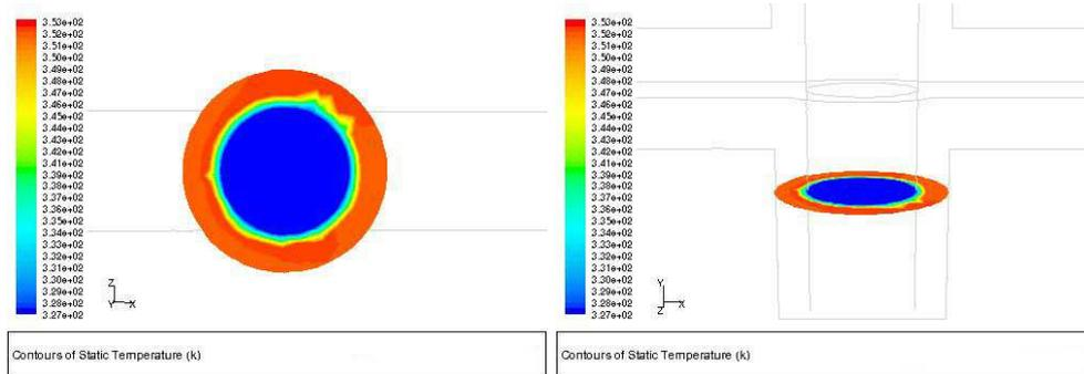
Fig. 2.16 Temperature distribution at section  $y = -15\text{mm}$
