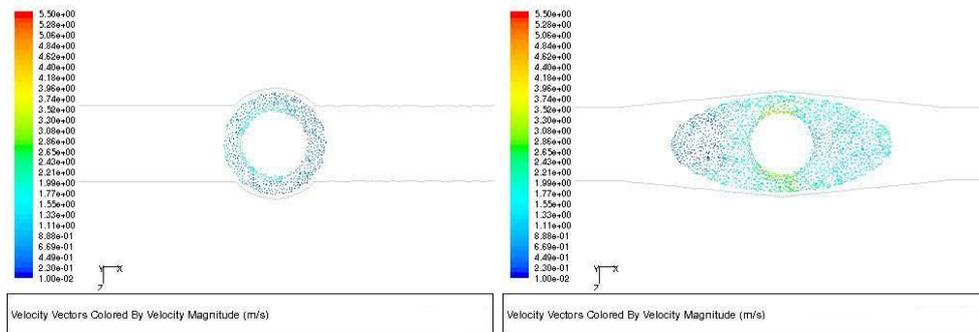
Fig. 4.12 Velocity vectors distributions at section  $y = -15\text{mm}$
