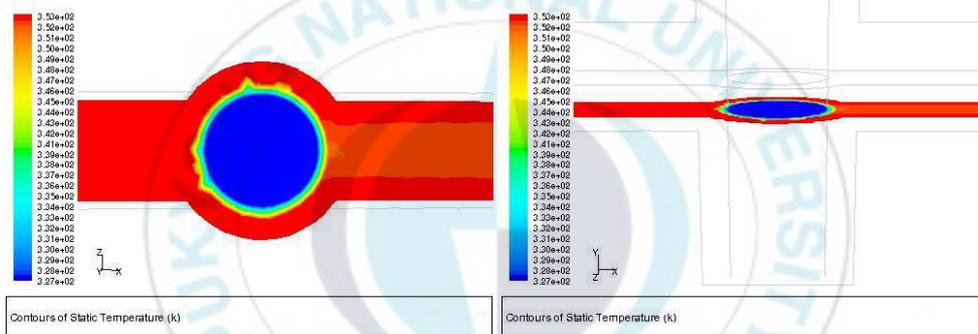
Fig. 2.14 Temperature distribution at section  $y = -5\text{mm}$
