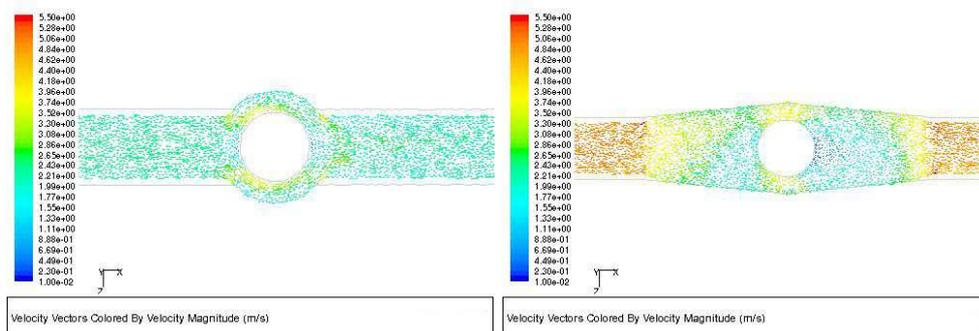
Fig. 4.8 Velocity vectors distributions at section  $y = 5\text{mm}$
