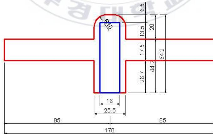
Fig. 2.1 Geometry dimensions of the present master joint model
