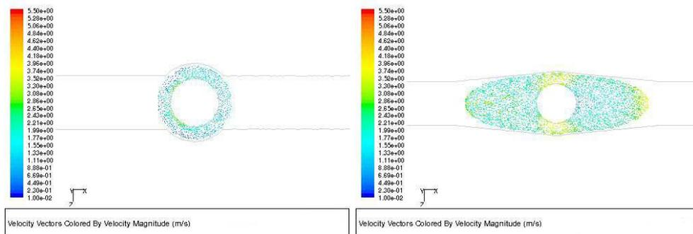
Fig. 4.11 Velocity vectors distributions at section  $y = -10\text{mm}$
