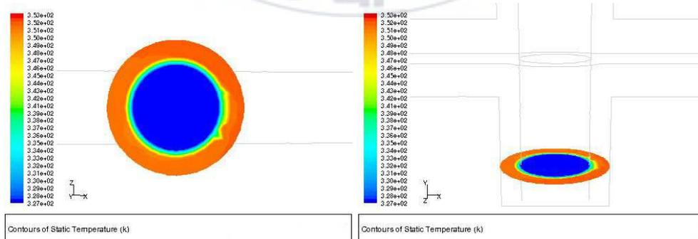
Fig. 2.18 Temperature distribution at section  $y = -25\text{mm}$
