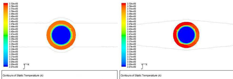
Fig. 4.26 Temperature distributions at section  $y = -25\text{mm}$
