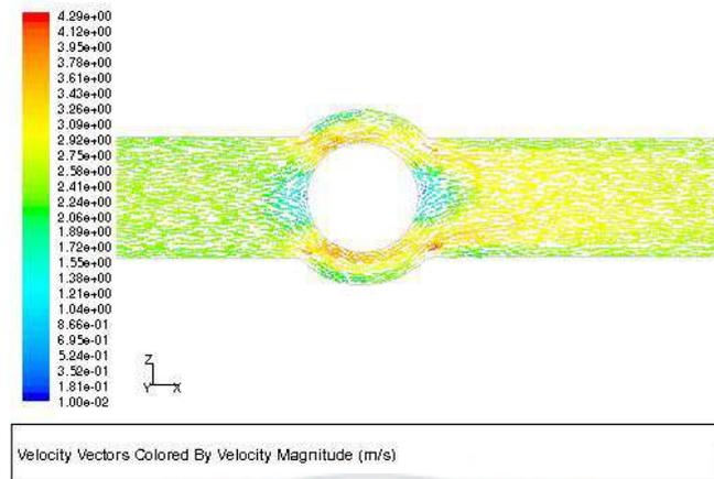
Fig. 2.4 Velocity vectors distribution at the central horizontal section ( $y = 0$ )
