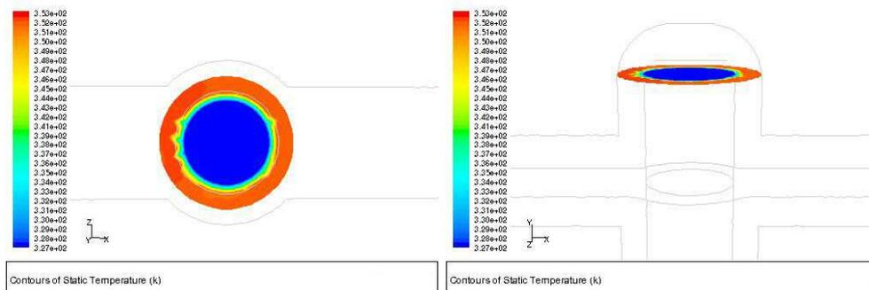
Fig. 2.9 Temperature distribution at section  $y = 20\text{mm}$
