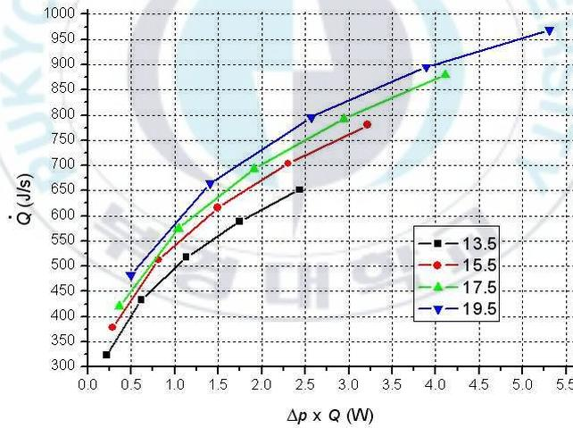
Fig. 3.12 Pump capacity  $P$  (W) vs. heat transfer rate  $\dot{Q}$  (J/s)
