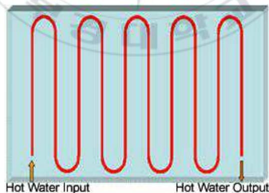
Fig. 1.1 Conventional floor heating system
