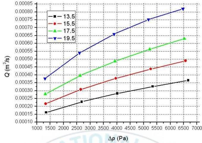
Fig. 3.10 Pressure difference  $\Delta p$  (Pa) vs. flow rate  $Q$  ( $\text{m}^3/\text{s}$ )
