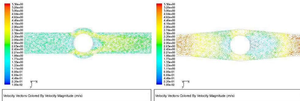
Fig. 4.9 Velocity vectors distributions at section  $y = 0$
