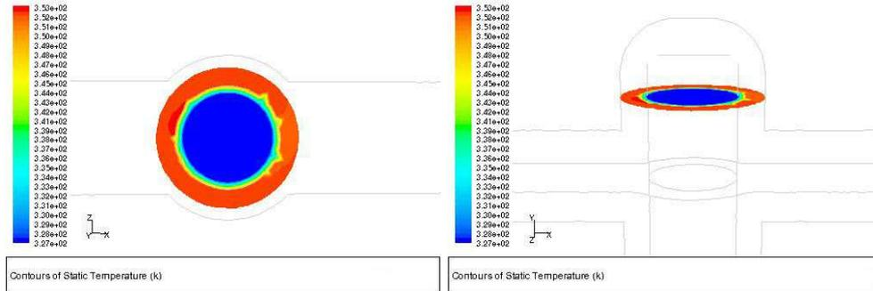
Fig. 2.10 Temperature distribution at section  $y = 15\text{mm}$
