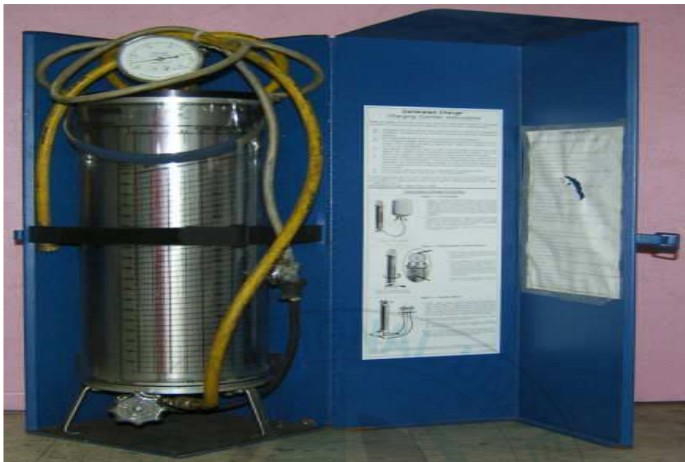
Fig. 16 Refrigerant charging cylinder
