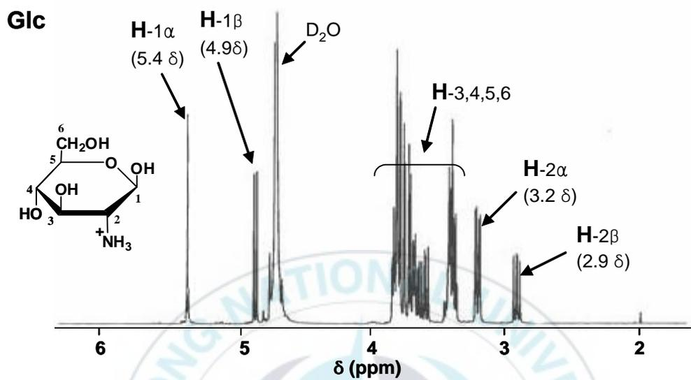
Fig. 3A.  $^1\text{H}$  NMR ( $\text{D}_2\text{O}$ , 400 MHz) spectrum of Glc.
