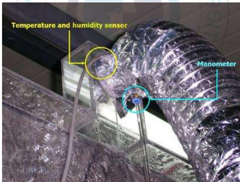
*Fig. 2.3.2 Photograph of measuring instrument at exit of system*
