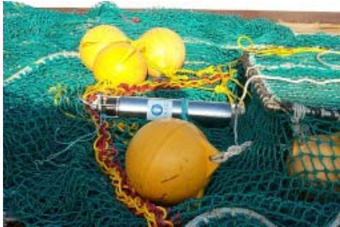
Fig. 3.2. The view of Acoustic Releaser attached to the trawl.
