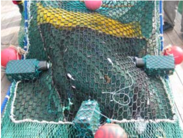
Fig. 5.6. Photo of underwater camera and lights attached to the Trawl Escapement Net.
