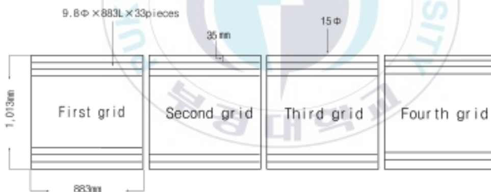
Fig. 3.1. Schematic view of Trawl Escapement Device (TED) for Grid panel type.
