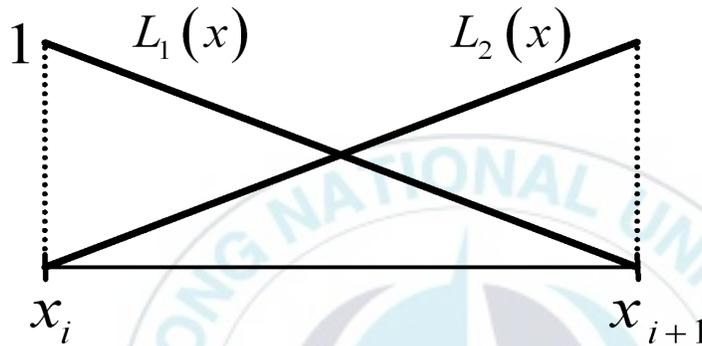
Fig. 3.2 Graphs of linear shape functions  $L_1$  and  $L_2$ .
