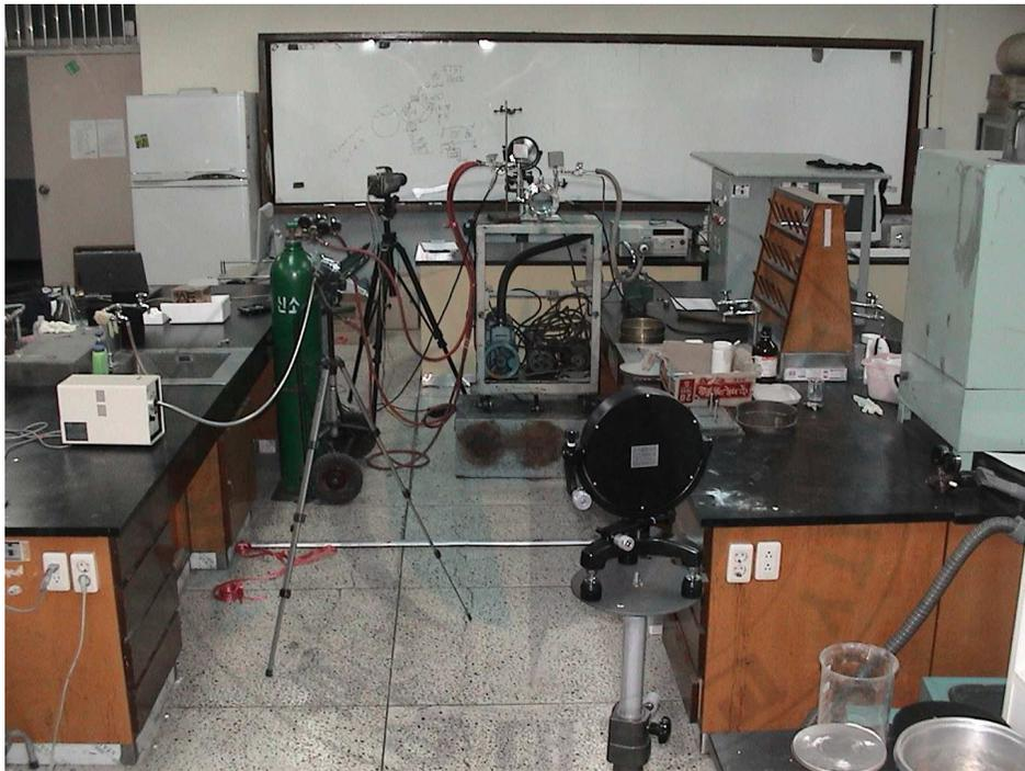
Photo 3 The picture of shadow photographing techniques for explosion appearance.
