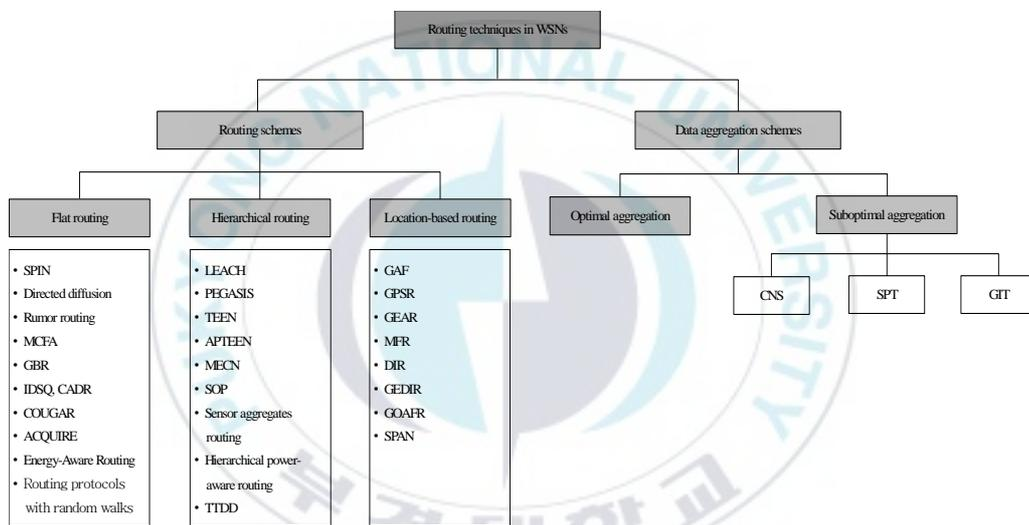
Figure 3. Routing techniques in WSNs
