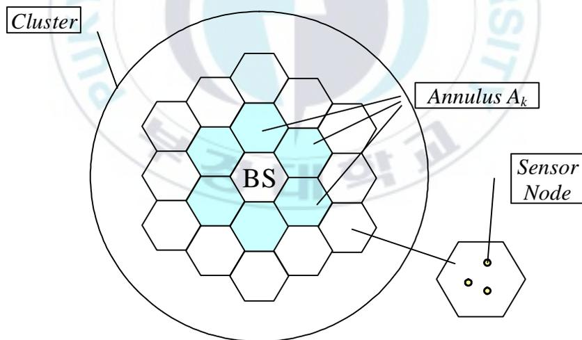
Figure 5. Hexagon tessellation model for each cluster given in Figure 1
