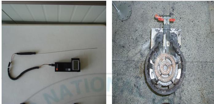
Fig. 3 Photograph of the thermocouple and burner
