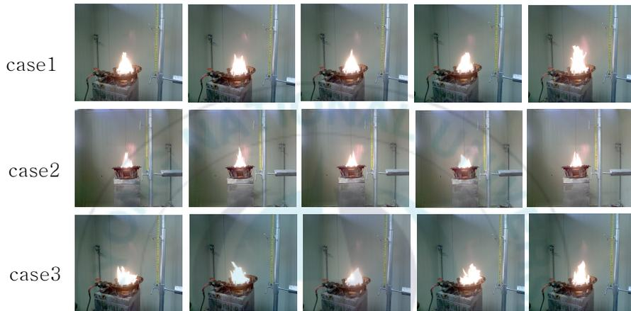
Fig. 32 Photographic of flame for fire size 7.1kw
