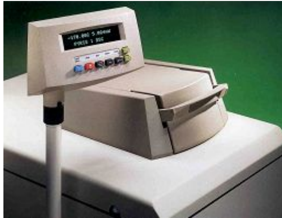
Fig. 11 DSC (Differential Scanning Calorimeter)
