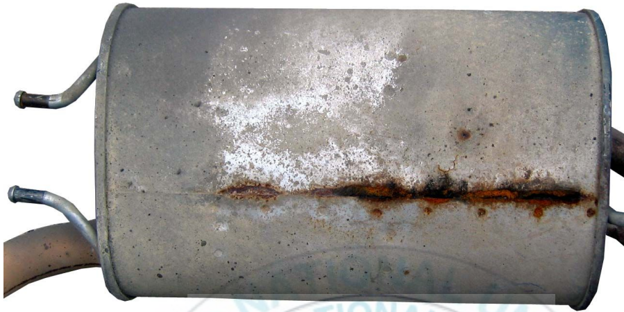
Photo. 1 Appearance of corrosion damage of muffler
