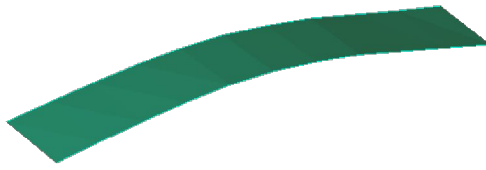
(a) Mode 1 (1st Bending)
